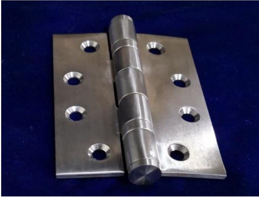
After 96 hours salt spray test,material: ss304
